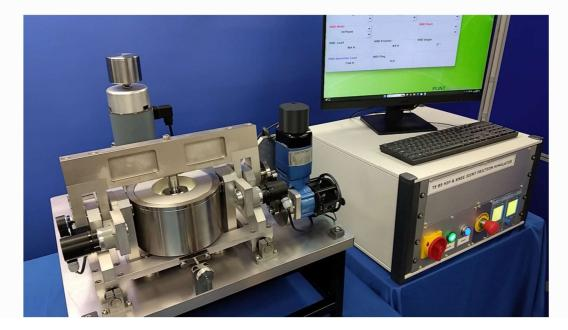
Control and data acquisition are implemented via host PC running COMPEND 2020 Windows compatible software, in conjunction with a Phoenix Tribology USB micro-controller interface.
