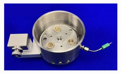
This adapter uses slipper shows taken from an actual radial piston pump and is used for evaluating both pump materials and hydraulic fluids.
