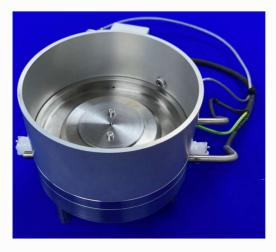
This adapter is for immersed (non-circulating) lubricant tests. In addition to the standard heaters, the assembly incorporates cooling passages that can be connected to a laboratory chiller.
