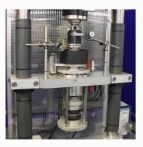
The precision low load adapter comprises a fixed cross beam, with pneumatic bellows and an integral air bearing, allowing precision low load tests to be run at loads down to 1 N. The maximum load is 1000 N.
