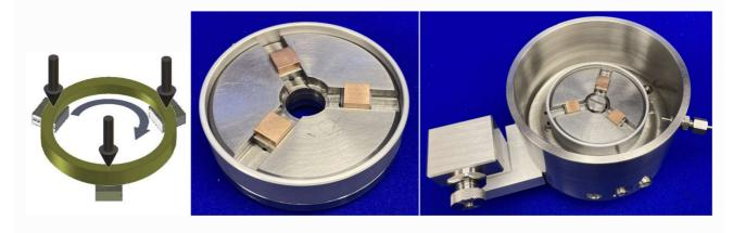
The adapter comprises three taper/flat-land pad specimens, which act in the same way as a conventional taper/flat land thrust bearing. The adapter allows Stribeck curves to be generated in under ten minutes, with less than 250 ml lubricant sample.
