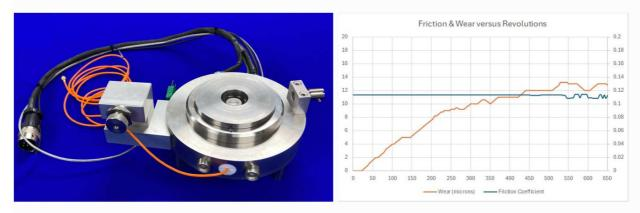
TE 92/AREA-D Specimen Mount with Capacitance Wear Sensor & Shaft Hub for Dry Tests
