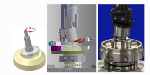
This adapter applies an axial load to a spherical bearing seat, which is subjected to orbital, as opposed to rotary, motion. Such bearings include hip joints and spherical radial bearings, under certain operating conditions.
