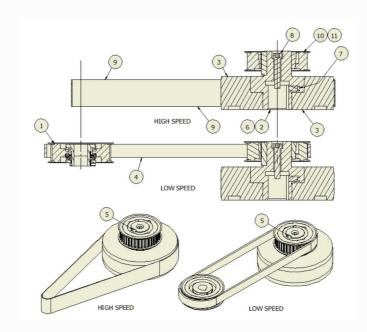
A high speed machine with 2.2 kW motor and single-phase supply and timing belt drive and torque limiter for speeds from 0 to 3,000 rpm, high speed flat belt drive for speeds 0 to 10,000 rpm. The test spindle main bearings are a matched pair of super-precision angular contact bearings and the maximum design speed is 10,000 rpm.
