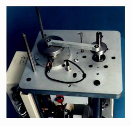
The TE 92/O Oscillating Drive Adapter converts machine to oscillating. The angle of oscillation can be set between 0 and 90° with limits on the maximum frequency at large angles. The drive comprises a crank mechanism connecting the motor output shaft to the test spindle.
