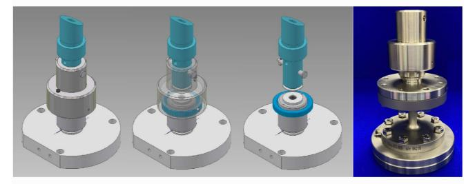
In this adapter, an upper chamber with a lip seal is rotated against a fixed shaft and the friction torque measured. The upper chamber is filled with lubricant and is thus the wet side of the seal. There are two advantages with the arrangement, firstly, thermocouples can be inserted into the non-rotating shaft to measure temperature of the material under the seal, secondly, it is easy to spot if and when the seal begins to leak.
