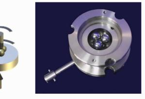
This comprises a test reservoir and precision polished test race. In this case there is no torque measurement. The adapter may be used in conjunction with **TE 92/2 High Load Actuator** to perform tests in accordance with:
