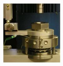
TE 92/FOUR/1 Sliding Four Ball Test Assembly
