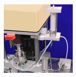
The system comprises a heated upper header tank, a lower sump tank and a peristaltic pump. The header tank is clamped to the right-hand machine column, which allows its height to be adjusted relative to the test assembly. Feed to the test adapter is by gravity, via a manual control valve and through a port which discharges in the centre of the adapter, with drain back to the sump tank, under gravity.
