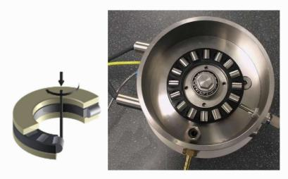
This adapter uses one half of a standard size 81208 TN roller thrust bearing, loaded against a flat lower disc sample, of chosen material. The standard bearing cage is used to locate the rollers, with the cage centred by a spindle mounted deep groove ball bearing.
