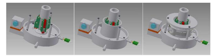
The adapter incorporates a fixed section of liner, which forms the specimen bath wall, and a rotating ring sample carrier. Lubricant may be dripped down the wall of the liner section, which is heated with a band heater.
