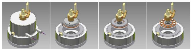
This system is designed to model Electrically Induced Bearing Damage (EIBD) and Electrical Discharge Machining (EDM). It includes a variable voltage source connected, via brush gear, to a commutator, so that the pulse always occurs at the same circumferential position.
