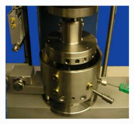
This is a test bath and shaft hub, for lubricated tests. It is used with any of the six current tooling inserts. The bath has a central port for lubricant feed and drain ports at different levels. It incorporates cartridge heaters and thermocouple for specimen heating and temperature measurement.
