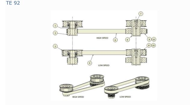
A standard speed machine with 2.2 kW motor, single-phase supply and timing belt drive and torque limiter for speeds from 0 to 3,000 rpm and Poly-V belt drive for speeds 0 to 6,000 rpm. The test spindle main bearing is a taper roller bearing with maximum design speed of 6,000 rpm.
