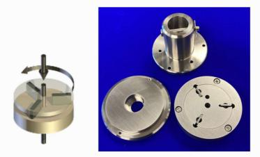
The tooling is used in conjunction with **TE 92/AREA-L** and comprises a non-rotating three-vane specimen carrier in contact with a rotating flat disc. The vanes are independently electrically insulated allowing electrical contact potential measurements to be made between each vane and the rotating disc.
