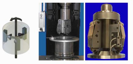
Instead of running up and down the liner, the ring samples are run around the internal circumference of a section of liner in either continuous rotation, allowing high sliding speeds to be achieved, or oscillating motion.
