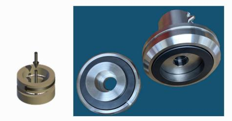
The tooling is used in conjunction with **TE 92/AREA-L** to perform tests using small-scale LVFA friction material test samples and for face seal testing. This tooling is normally customised to meet client specific requirements.
