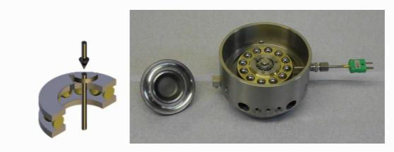
This adapter uses one half of a standard size 51208 68 mm O/D 40 mm I/D thrust bearing, with the balls running between the normal bearing race and a flat disc. A cage is provided to retain the balls.
