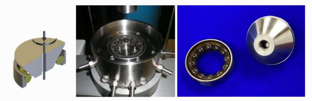
This adapter uses the lower race and cage of a standard angular contact bearing (SKF 7206), with the inner race replaced by a conical specimen. The cone angle is such that the rolling contact is pure rolling with no spin. With silicon nitride balls in the bearing race, contact pressures up to 5.5 GPa can be achieved. The cone is subjected to the highest number of contacts and thus it is the rolling fatigue performance of the cone material that is investigated in this test configuration.
