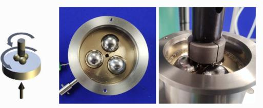
This adapter is for running rolling four ball tests with inch balls, separated by a cage.
