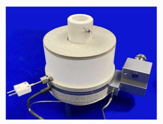
This is a high temperature specimen mounting for dry tests using either three pin-on-disc or thrust washer tooling.
