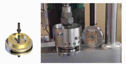
The tooling is used in conjunction with **TE 92/AREA-L** This adapter comprises a shaft mounting collet for carrying cylindrical tube specimens, which have precision ground ends, and a fixed specimen mount, for square coated plate specimens. Radial grooves machined in the plate specimens allow lubricant entrainment, with lubricant supply via the bath central feed port.
