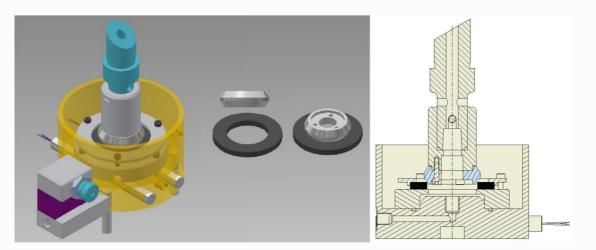
This adapter is designed for testing the frictional properties of rubber materials for seals. A rotating steel cone is axially loaded against a ring made from rubber sheet. Tests can be either dry or lubricated.
