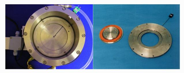
The test bath includes both cooling passages for removal of heat with cooling fluid during low temperature tests and resistance heaters for adding heat for high temperature tests.
