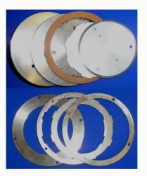
The rotating specimen is mounted on a flange using a modular clamping system to accommodate a range of diameters and spline arrangements. Parts of the clamp are manufactured to suit the spline arrangements on the rings.
