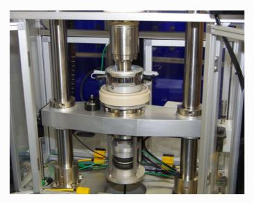
For tests at temperatures above ambient, a separate heated test assembly is provided. This incorporates an aluminium heater block with an electrical band-heater and includes an NC-DVRT sensor for wear displacement measurement. The assembly allows tests to be run at temperatures up to  $150\ ^{\circ}\text{C}$ .
