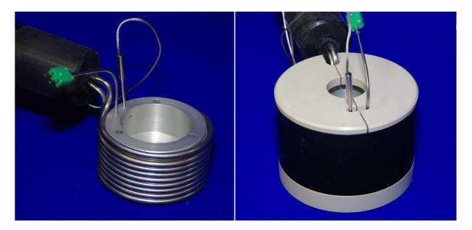
A unique feature of the cooling system is that, unlike more conventional systems, it does not involve the use of a pumped heat transfer medium. Instead, the refrigerant from a standard laboratory chiller is delivered, under pressure, to the test assembly, where it is expanded in a cooling coil, which is wrapped around an aluminium cooling block. This provides a very efficient means of cooling, having eliminated the heat transfer and pumping losses associated with using a heat transfer fluid.
