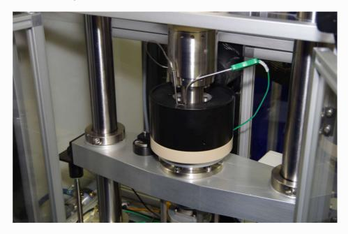
The refrigerated test assembly mounts on the bellows actuator shaft, which projects through the air bearing, with the bulky refrigerant pipes projecting through the rear of the test enclosure. The rotating specimen, mounted on the lower end of the in-line transducer, projects downwards into the refrigerated assembly.
