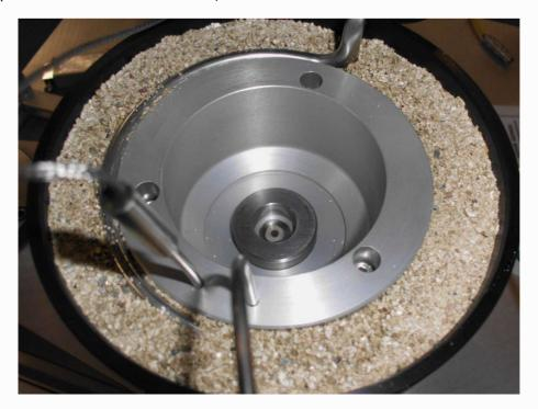
An NC-DVRT sensor is mounted in the centre of the cooling block, to measure the gap between the lower specimen assembly and a target on the upper specimen shaft, a reduction in the gap providing a measure of specimen wear. In order to avoid icing in the test assembly, an enclosure is provided, fed with compressed air via a desiccant dehumidifier tube.
