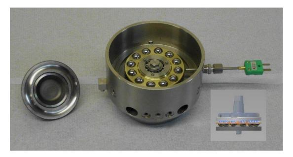
Unlike the ARKL test, our adapter uses just one race from the 51208 bearing, with the lower race replaced by a flat disc and the balls retained by a special cage. The spin induced between balls and flat disc promotes fatigue failure.
