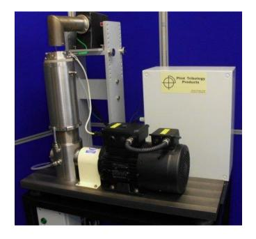
Valve seat recession is dependent on the velocity of the valve at impact with the seat. Clearly, the velocity of the valve at any part of the cycle is of no relevance. It follows that using a standard automotive, variable velocity cam, to generate the motion, will require very precise adjustment of the relative position of valve and seat, in order to achieve the required impact velocity. As wear occurs, the position of impact, relative to the motion, will change and hence the velocity of impact.
