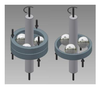
We are developing a ball on rod rolling contact fatigue adapter for use with the <u>TE 92</u> and <u>RCF 2</u> test machines. We may also offer the adapter as part of a free-standing test machine.
