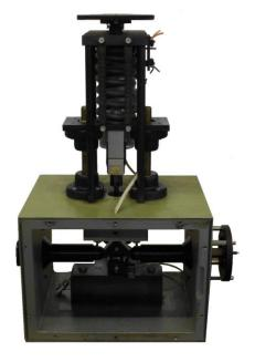
The guts of the machine comprises a test enclosure in which is mounted the heated, fixed specimen assembly. The fixed specimen is mounted on a standard Kistler 3-axis piezo transducer, of which only one measuring axis is used, this to measure friction. The loading system incorporates a spring and screw actuator mechanism driven by a standard servo motor and incorporating a standard Interface strain gauge force transducer, for load feedback.
