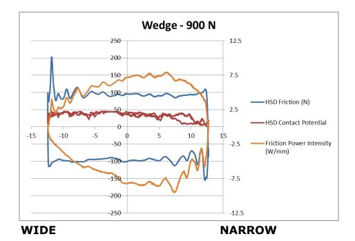
The resulting friction power per unit width is naturally skewed towards the narrow end of the wedge sample for both directions of motion.
