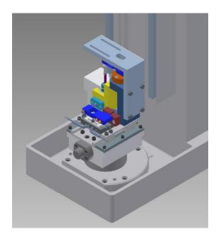
The new reciprocating drive assembly uses the same scotch yoke cam system as on the standard TE 77 High Frequency Friction Machine, a drive system with proven longevity.
