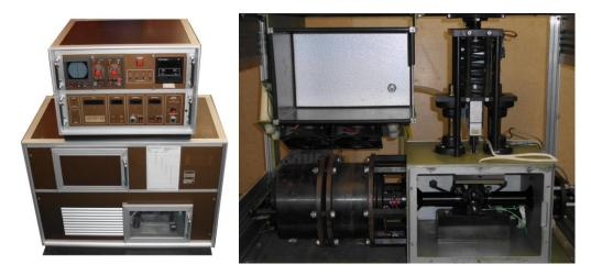
We decided that it did not make sense to attempt to re-use or replace the expensive and very heavy electro-magnetic drive system and that the right solution was to replace this with a simple, low cost, fixed stroke, motor driven reciprocating drive.
