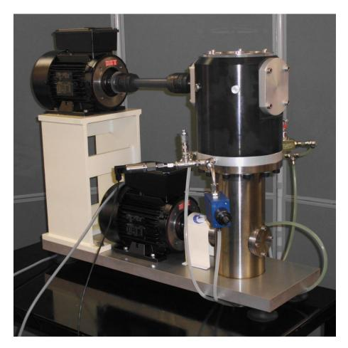
The prototype pulse actuator bearing fatigue rig is now under test. The theoretical force generated by the current actuator, which has a diameter of 125 mm, is 1227 N per bar. The current unit produces a peak force of approximately 47 kN. The design is fully scalable and can be adapted for testing both plain and rolling element bearings. Click on the link to view the YouTube video.
