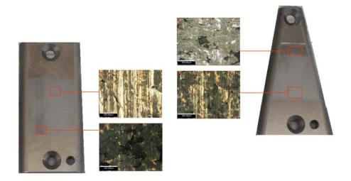
One of the interesting features of these experiments is that they successfully demonstrate the lack of connection between friction and wear. Furthermore, they demonstrate that with these particular experiments, friction is independent of apparent area of contact, the friction being independent of contact width.
