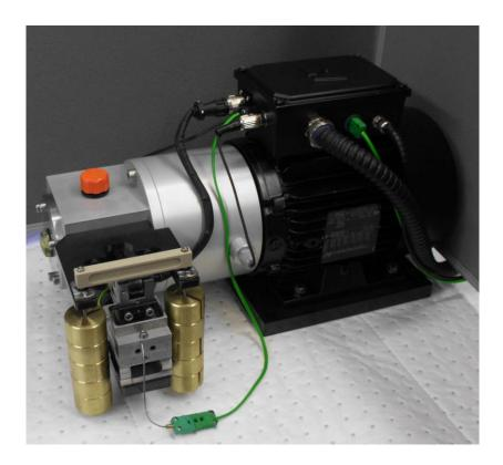
We are currently assembling a modified fuel lubricity tester, designed to run at higher loads and longer strokes than those specified in the diesel fuel lubricity test standard, allowing tests to be performed with a sliding line contact as opposed to a less sensitive sliding point contact. Key specifications are:
