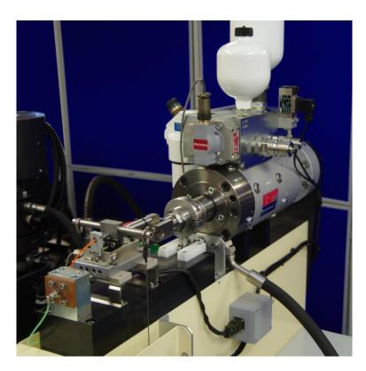
We have updated the design of the DN 44 to incorporate a new hydrostatic bearing servo hydraulic actuator and to replace the manual loading system with servo controlled loading.
