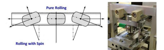
The original purpose of the adapter was to model the sliding-rolling contact in a Tripod CV joint. A short video on this experiment can be viewed on our LinkedIn page. Click on the link to see <u>Tripod CV Joint Friction Test</u>.
