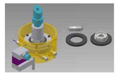
We have completed the design and manufacture of cone on elastomer ring tooling for dry and lubricated friction tests of metal-polymer contacts.
