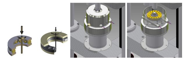
For a number of years, Professor Jorge Seabra and his team at the University of Porto have been publishing the results of tests on a modified TE 92 machine, with a rolling bearing test assembly mounted direct on a torque transducer. The most recent paper appears to be <u>Friction torque in grease lubricated thrust ball bearings</u> - T Cousseau, B Graca, A Campos, J Seabra - Tribology International 44(5):523-531 2021.
