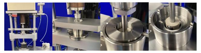
We have now successfully run a standard ball on rod rolling contact fatigue test geometry, on a TE 92HS, for extended periods, at 10,000 rpm.
