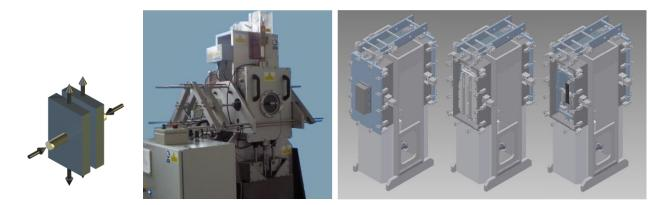
We are completing the re-design of the TE 104 test rig, improving the hydrogen security, increasing the test pressure to 5 bar, the load to 500 N and the stroke amplitude to +/-100 mm. Maximum frequency remains 20 Hz and instrumentation includes on-line measurement of friction, wear displacement and specimen surface temperature on each of the four tests stations.
