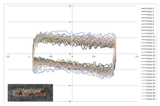
For this ball on flat test, the stroke was 2 mm and the load was 150 N.
