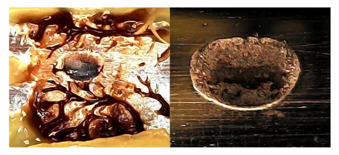
Our initial tests were run with the ball specimen running in a curved groove. We then decided to see what would happen if we ran the ball against a flat surface, which is, of course, much easier to make than a grooved specimen.
