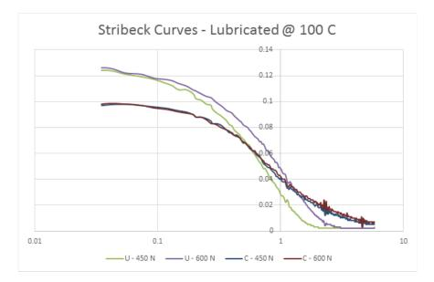
When it comes to curves with different materials, we begin to see some interesting behaviour. In this case, a coated and an uncoated test ring are compared, demonstrating much reduced friction in the boundary regime with the coated specimen, but delayed arrival at the hydrodynamic regime. Furthermore, in the hydrodynamic regime, the coated ring produces slightly higher friction than the uncoated ring.
