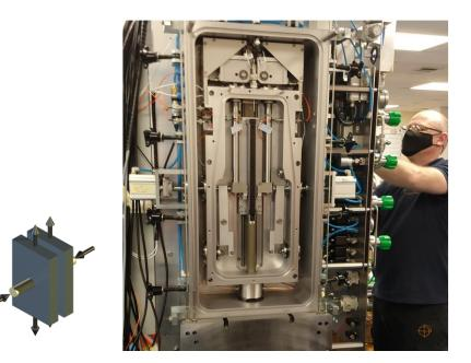
The first of the much modified and performance enhanced TE 104 High Speed Reciprocating Machine is currently being assembled. The four-station machine, designed to run at strokes up to 200 mm, frequencies up to 20 Hz and loads up to 500 N, comprises an inner hydrogen test chamber, rated to 5 bar pressure, inside an outer nitrogen chamber, rated to 10 bar. Instrumentation includes friction, wear and non-contact temperature sensors on each test station.
