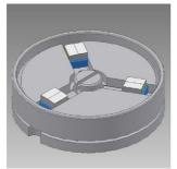
We have now optimised the taper wedge angle and surface finish of our taper land/flat land specimen pads, with encouraging results.
