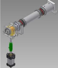
Production of the latest version of servo hydraulic, high load, low speed, journal bearing friction and wear tester is under way.
