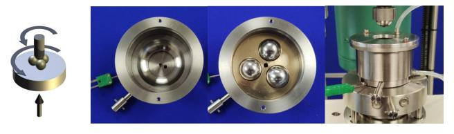
With balls larger than the standard 1/2-inch balls, it is necessary to separate the three lower supporting balls with a cage, to prevent excess friction between the balls. Large diameter rolling four and five ball adapters have been designed with contact angles in the range 40 to 50 degrees. With this design, a contact angle of 45 degrees has been chosen; this simplifies the arithmetic, when calculating the contact load.
