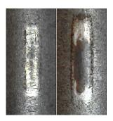
Fretting corrosion can be seen on both specimens, with more severe damage on the right specimen.
