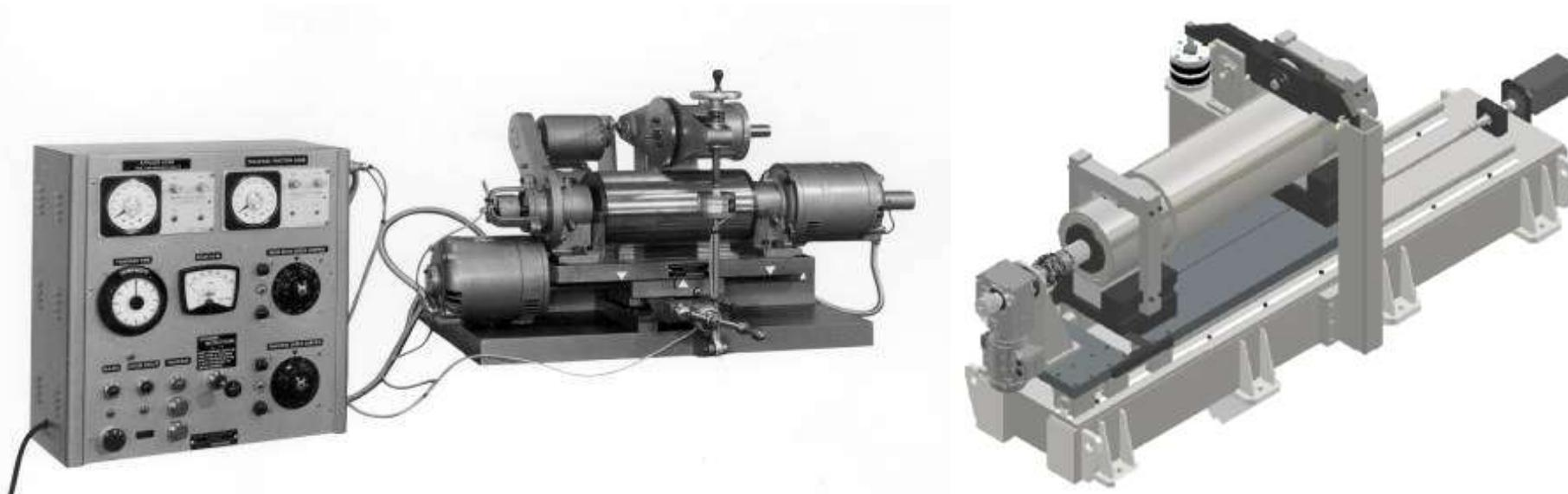
The original traversing roller on drum machine was designed by Plint and Partners Ltd for British Rail Research in the 1960s. The roller is not driven but is free rolling against the drum. Indexing the drum relative to the roller generates skew in the contact, with the resulting axial force measured by a transducer connected to the drum. Sixty years on, we have been asked to design and build an updated version of the rig.
