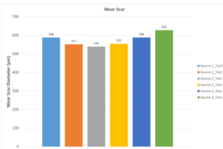
The friction coefficient results are all within the specified repeatability range: difference between successive results not exceeding 0.008. The wear scar diameters results are all within the specified repeatability range: difference between successive results not exceeding 70 microns. We will leave you to draw your own conclusions.
