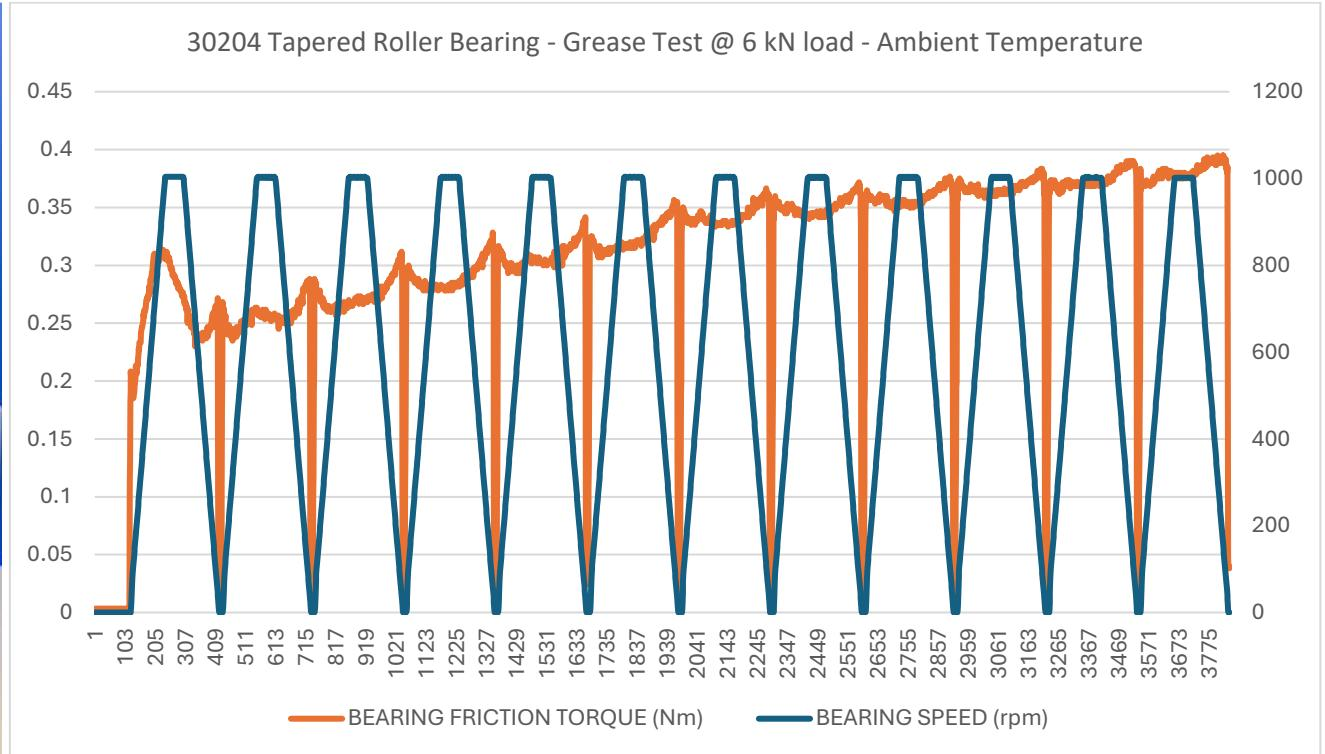
Testing with different grade greases is underway using angular contact and taper roller bearings, at loads and speeds relevant to wheel bearing applications. These tests are run at room temperature, with speed ramps used to generate torque-speed curves at different loads. To view a short video, click on the [link](#).
