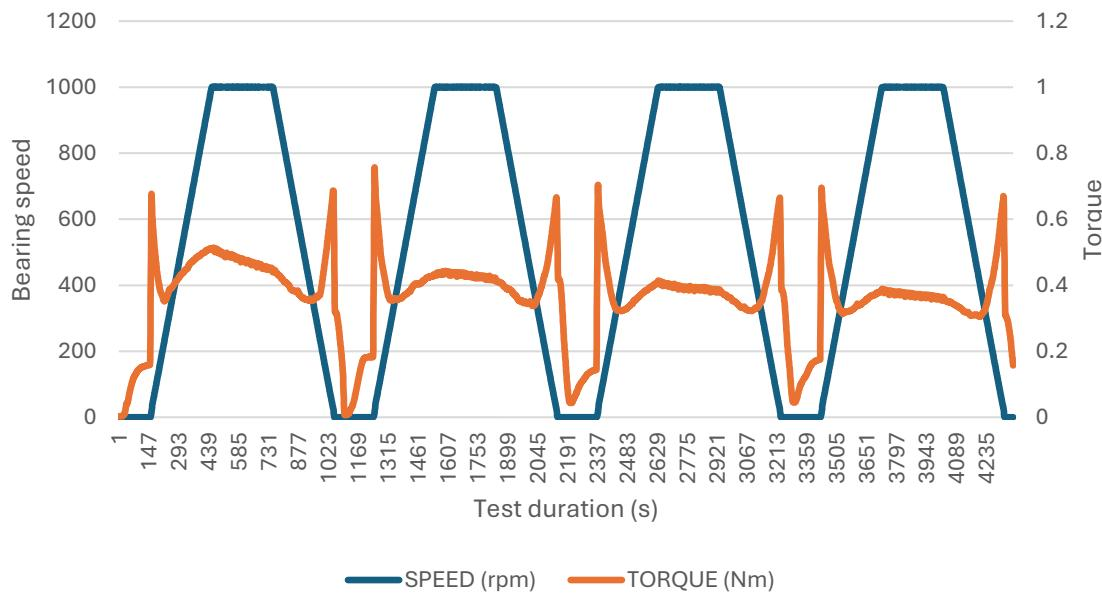
Data has been generated using our prototype tooling, producing some interesting results. Of note is the magnitude of breakaway friction, at start-up, particularly when testing axially loaded taper roller bearings. Longer term grease tests are planned, with the addition of hot air heating. We also plan to run lubricant shear stability tests, with on-line monitoring of friction torque.
