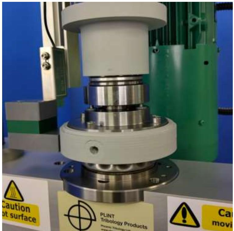
30204 TRB : Speed Ramp Test on EP Grease
