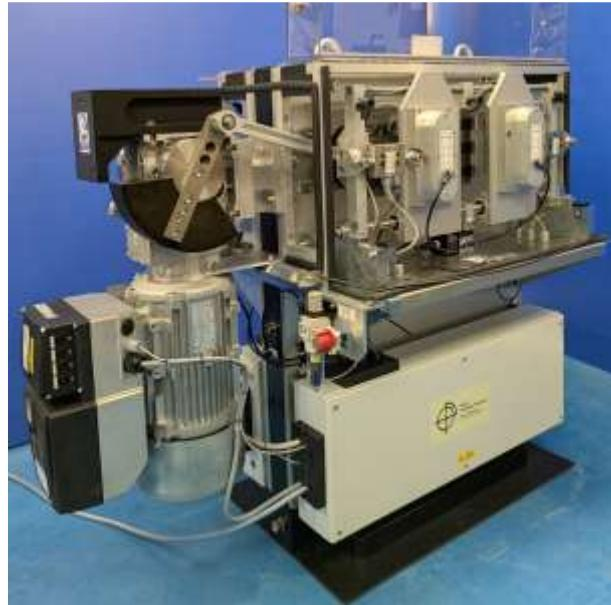
The latest unit of this twelve-station friction and wear machine has been delivered.
