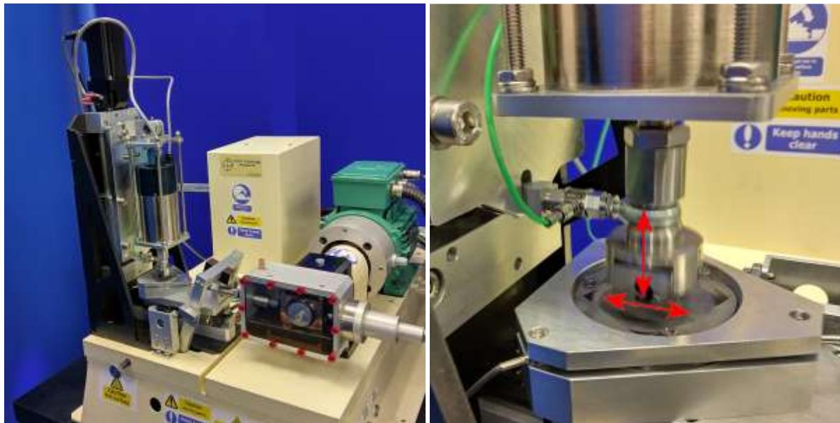
We have completed design, development and delivery of a new impact fretting adapter. To view a short video, click on the [link](#).
